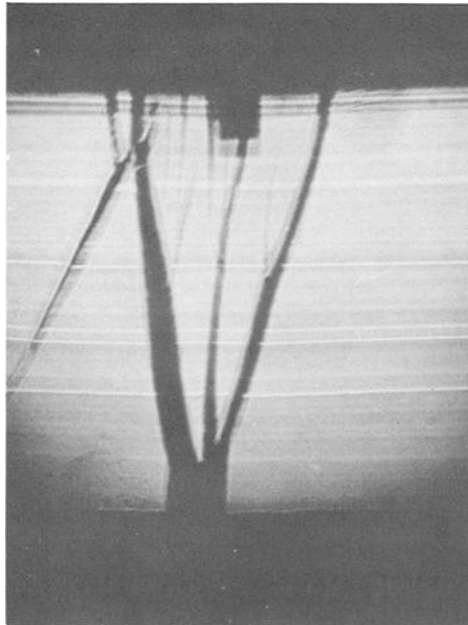
FIG. 8—Match in longitudinal striae as seen in the reflection image of several shards of fractured glass.
