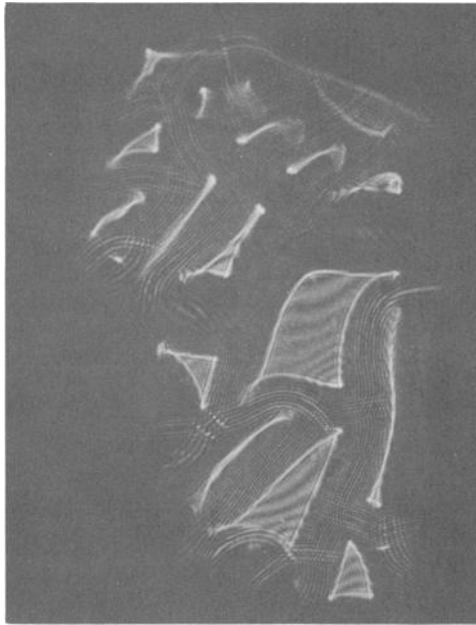
FIG. 9—Reflection image of an extensively crazed piece of disannealed glass.
